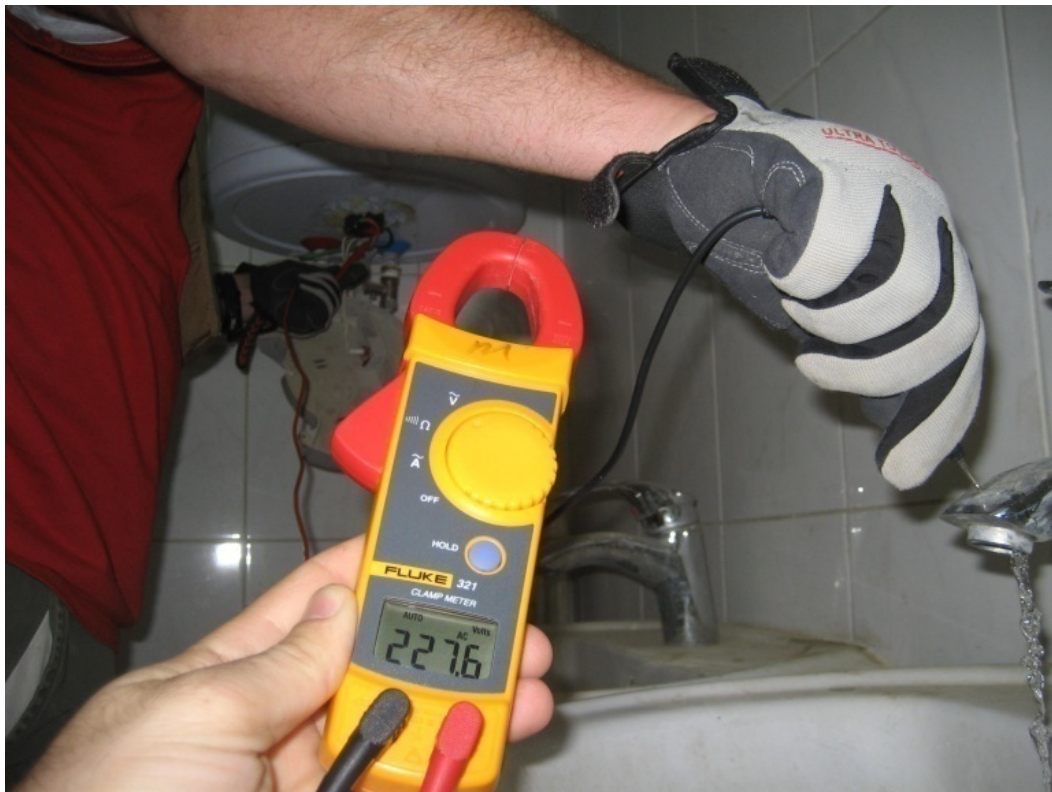
Figure 3—Photograph of voltmeter reading in water stream
