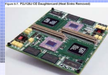
Figure 6-7. P2J128J CE Daughtercard (Heat Sinks Removed)
