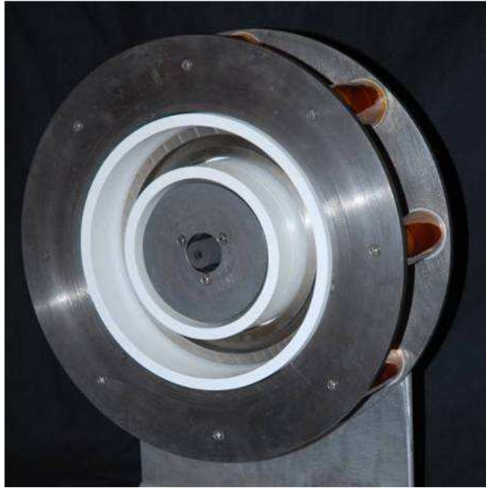
Figure 3-9 Photograph of the 6 kW laboratory Hall thruster with a centrally mounted LaB6 hollow cathode.
