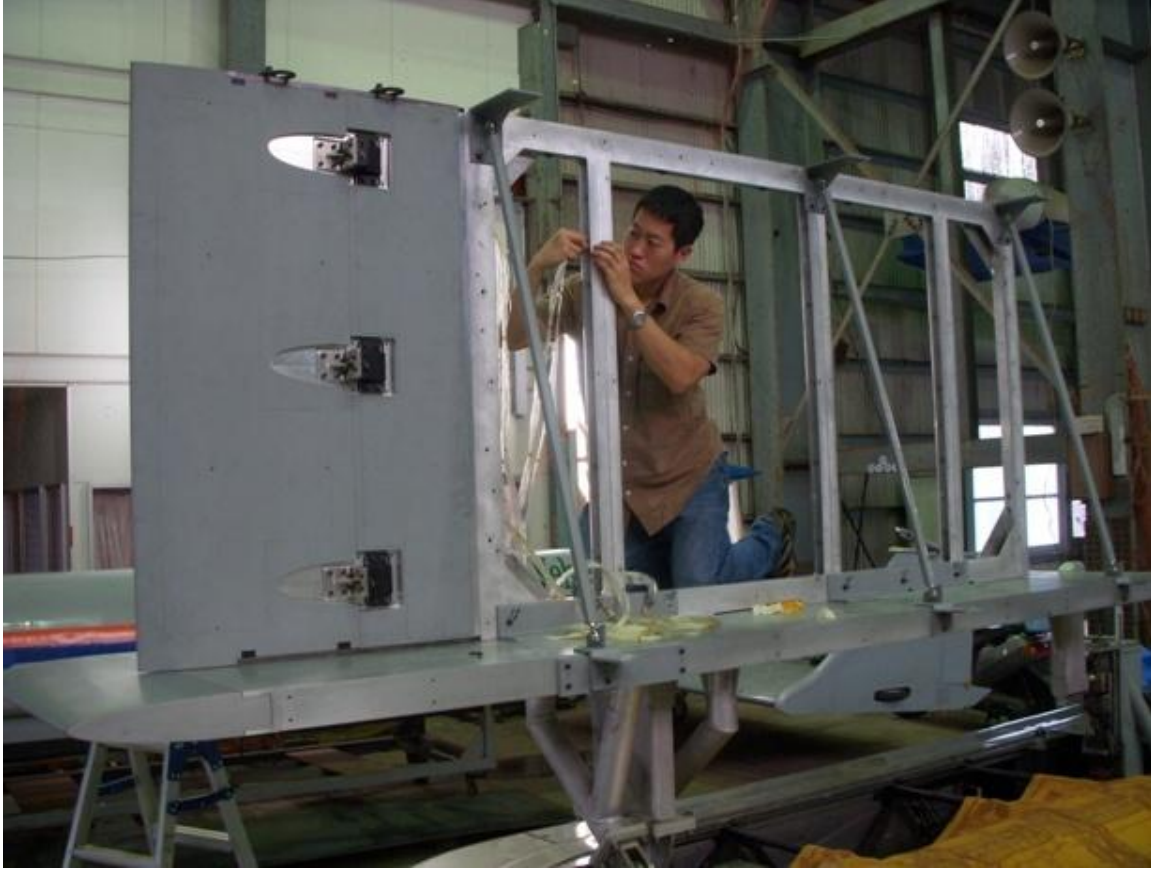
Figure 73: Gradient-Zero leading edge installed on common frame.
