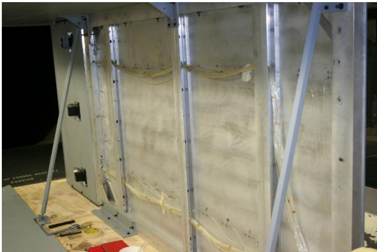
Figure 840: Upper and lower splitter plates installed; pressure routing complete.
