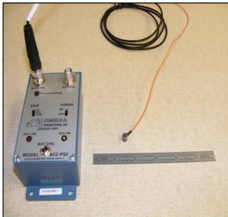
Figure 330: Accelerometer (right) and its power supply/amplifier (left).
