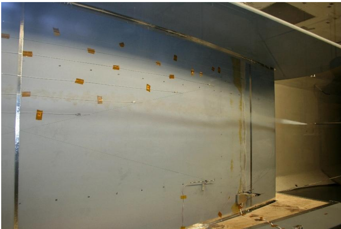
Figure 64: Smoke wand used on Gradient-A.
