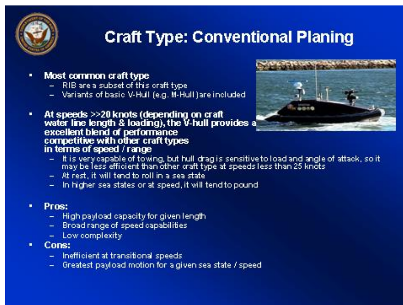
Figure 28 – Conventional Planing Hull Type
