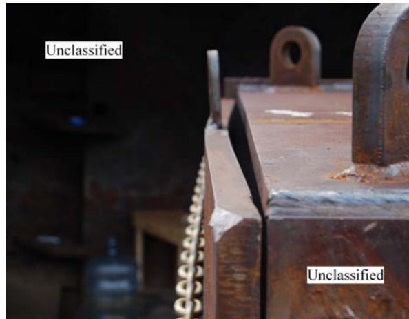
Figure 8.16. Confined blast post-test #2 post-test, chamber door deformation.
