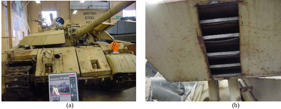
Figure 2.2. a) T55 Enigma armored Iraqi tank and b) close-up of spaced armor cross-section [Piggott, 2004]
