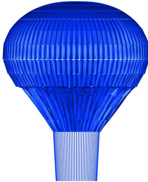
Figure 5.24: Parachute shape using a \tau_{REEF} value of approximately 13%: Stage 2 and under “symmetric FSI” conditions..
