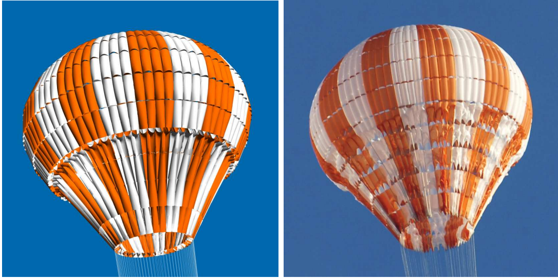
Figure 5.28: Comparison of results obtained using computational tools (specifically resulting from “symmetric FSI” and M2C SCFSI) to NASA provided drop test.
