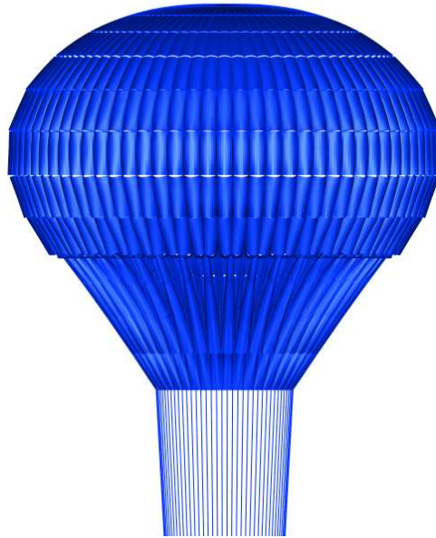
Figure 5.26: Parachute shape using a fine mesh and a \tau_{REEF} value of approximately 13%: Stage 2. This shape is obtained using SCFSI M2C technique.
