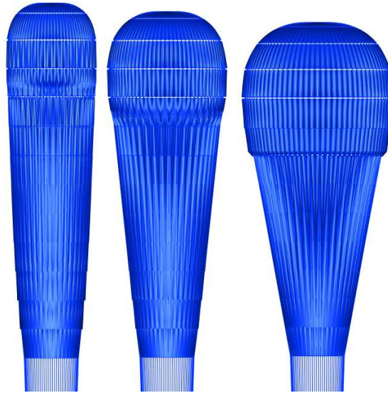
Figure 5.31: Parachute shapes using a \tau_{REEF} value of approximately 7%: Stage 1. Results from stand-alone structural mechanics computations where pressure profiles are generated to match shapes observed during NASA drop tests. From left to right, shapes show progression of shape during this reefed stage.
