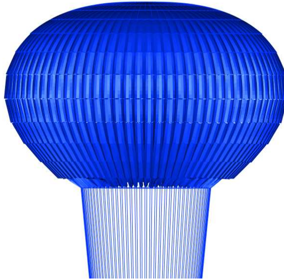
Figure 5.22: Parachute shape using a \tau_{REEF} value of 21.6% and under “symmetric FSI” conditions.
