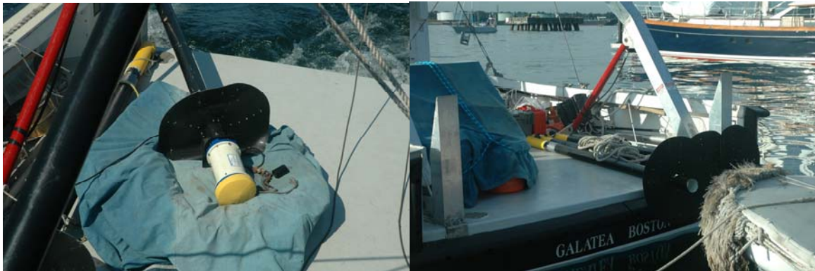
Fig. 1. Spars used for suspending instruments and dampening motion generated by surface waves. Top figure shows two spars in operation, holding the camera/velocimeter package (distant) and a 1200 kHz ADCP. They are tethered and cabled to the boat for real-time data display, but can also be cast free in internal recording mode. Lower left shows the bottom half of a spar with ADCP attached (sensors covered); lower right shows three spars on deck.
