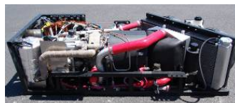
10kW Rotary JP-8 Auxiliary Power Unit
