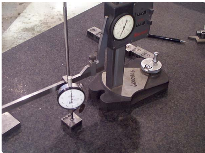
Figure 3. Dent Block Depth Measuring Device - Dial Indicators
