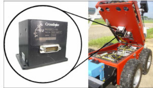
Fig. 1: ATRV-Jr mobile robot and equipped inertial measurement unit
