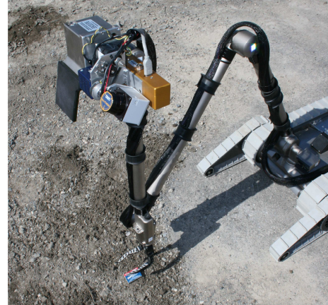
Figure 5: ASI's Packbot modified for 3D visualization.
