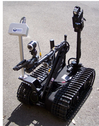
Figure 6: ASI's stereovision system mounted to the TALON robot using a quick-release bracket (silver camera on left of image).
