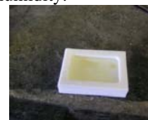
Figure 5. Poly(methyl methacrylate-co-1-butyl-3-vinylimidazolium bromide) (50mol% MMA) film dissolving in ionic liquid.
