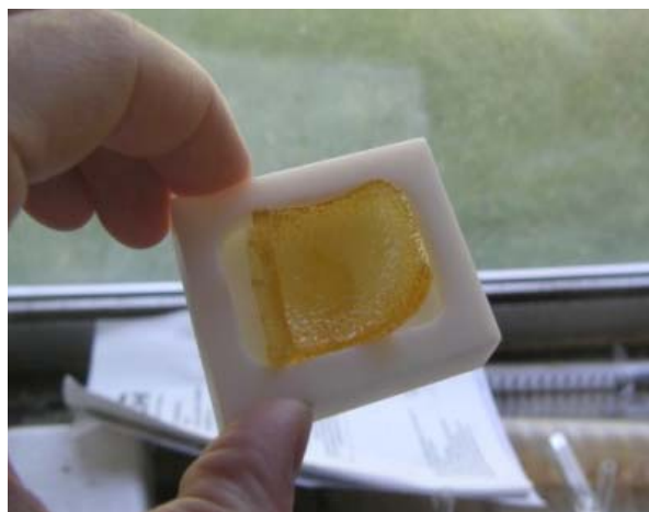
Figure 7. Photograph of BVIM-gel hydrated with humid air.
