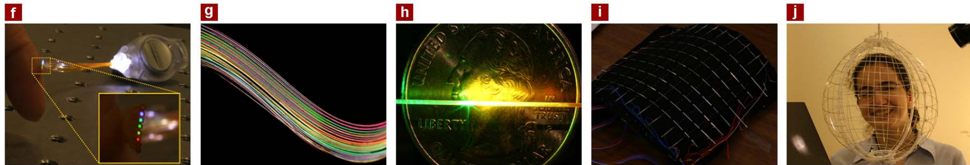
f Hollow transmission fibers g Optical cavity fibers h Surface emitting fiber lasers i Thermal detector fibers j Optical detector fibers
