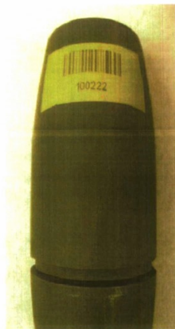
Figure B-10 Projectile showing no oxidation
