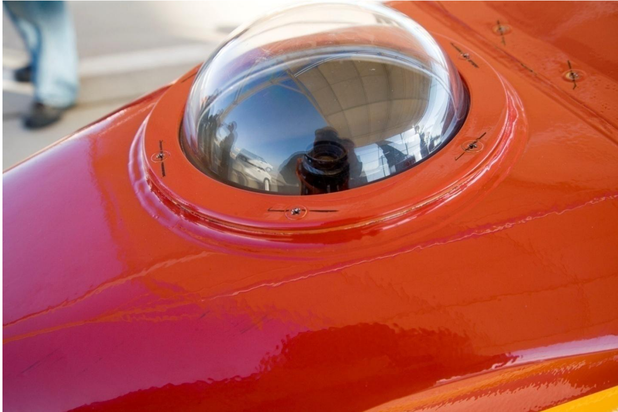
Figure B2: Video Camera Installation
