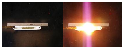
Figure 7 Frames from a video of the ignition of PSi-bismuth oxide (( courtesy, Dr. Puszyński and Chris Bulian South Dakota School of Mines and Technology (SDSMT))
