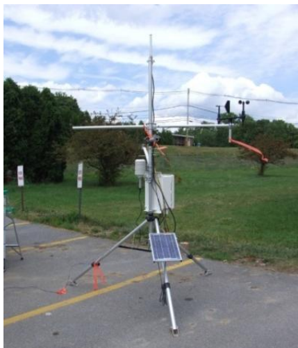
Figure 8. A base weather station. Meteorological measurements include air temperature, humidity, surface temperature, solar radiation, wind speed, and direction.
