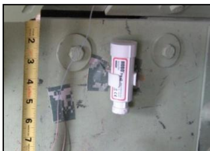
Figure 9. Temperature and humidity sensor (HOBO v2, Onset Computer Corporation, Pocasset, MA).
