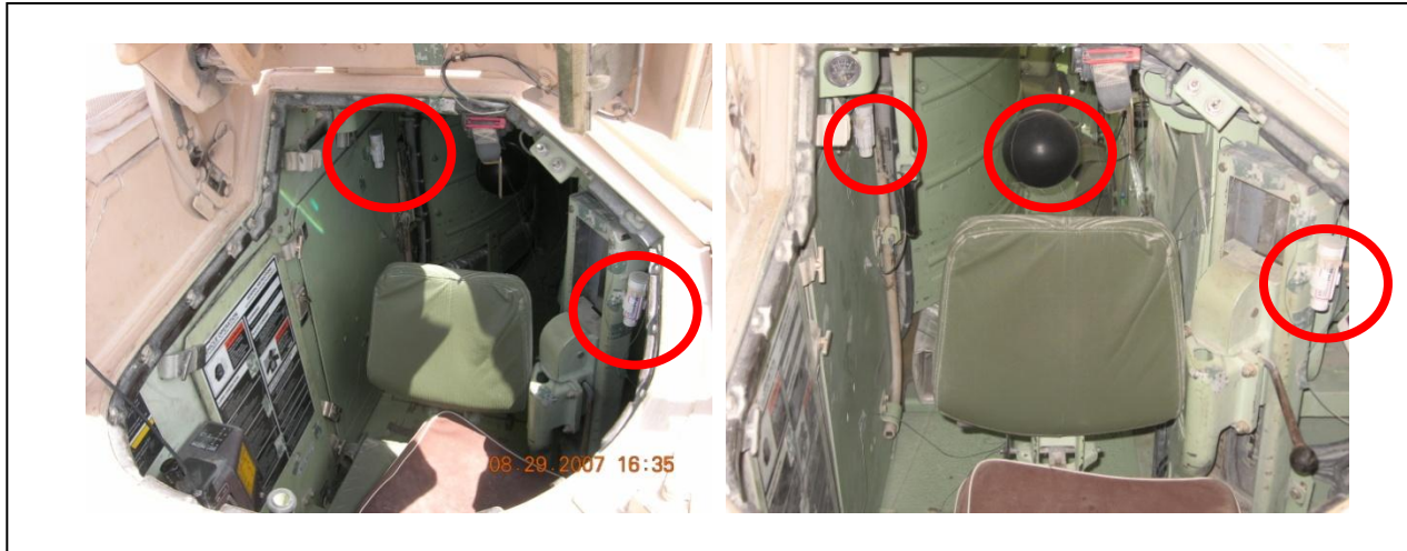
Figure 27. Two views of driver's compartment BFV with sensors in place. HOBO v2 are located on engine access panel to driver's right rear and left front at edge of hatch. Black globe is in passageway behind driver. Curved area behind black globe is the turret wall.
