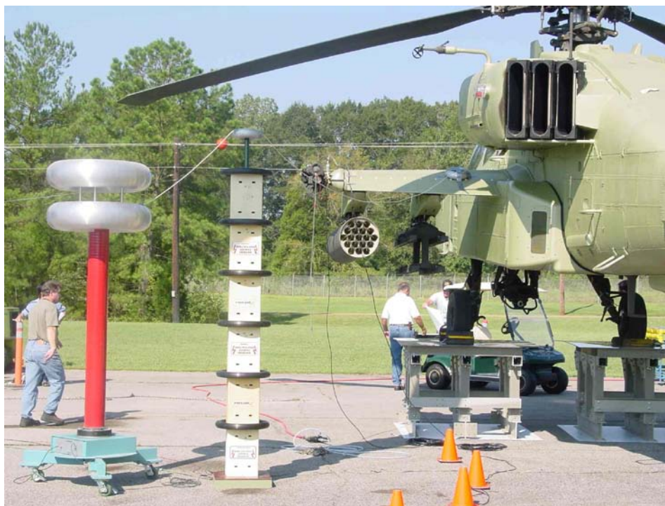
Figure F-4. Example P-Static Test Setup with Charge Generator & Voltage Divider.
