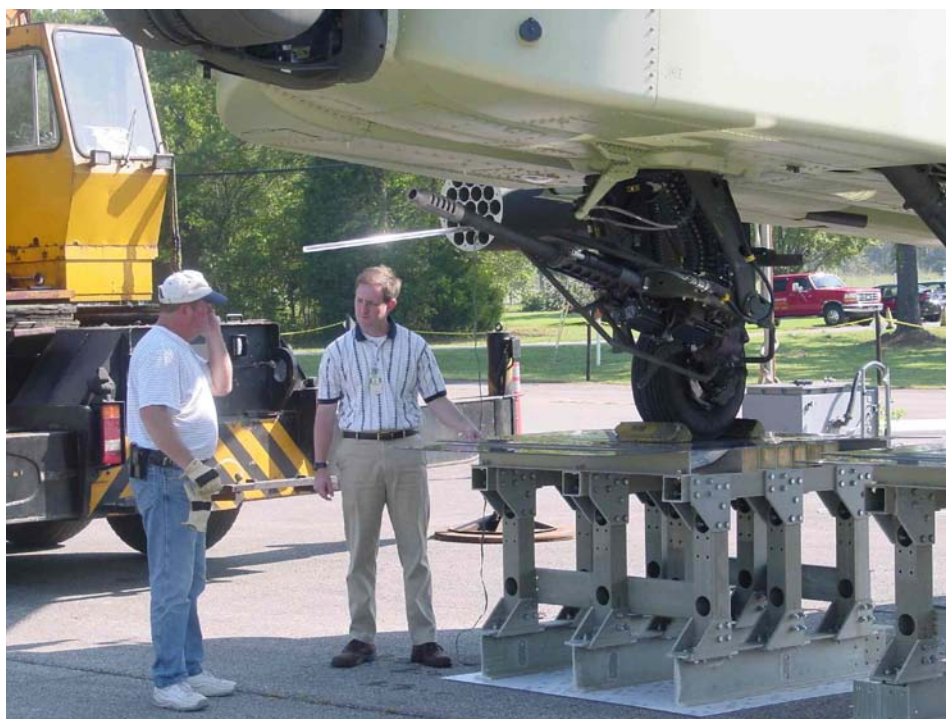
Figure F-5. Example P-Static Test Setup – Isolation Test Stand Close-up.
