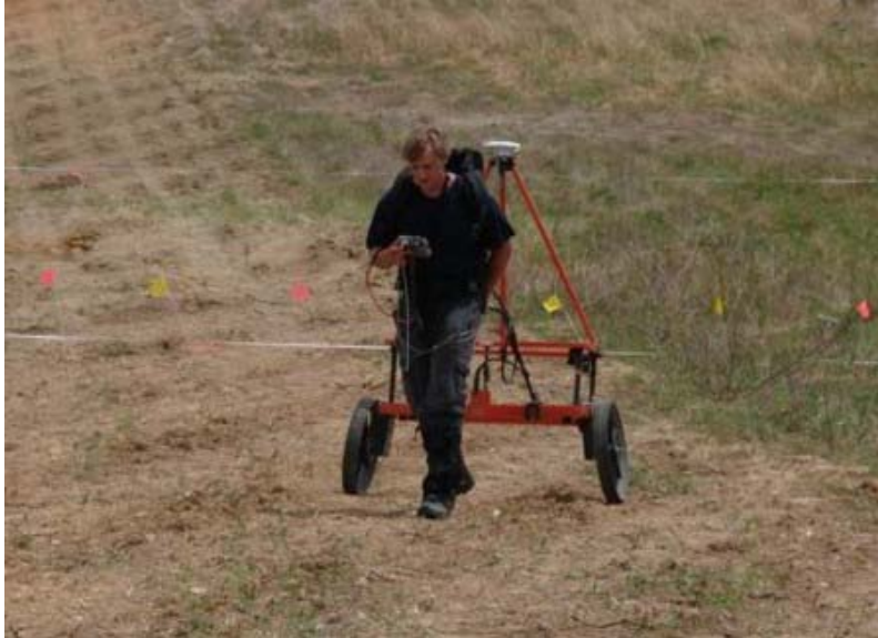
Figure 2.13: Photograph of the EM61 Cart collecting data at Camp Sibert.
