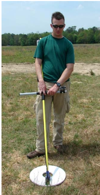
Figure 2.18: Photograph of the GEM Cued collecting data at Camp Sibert.
