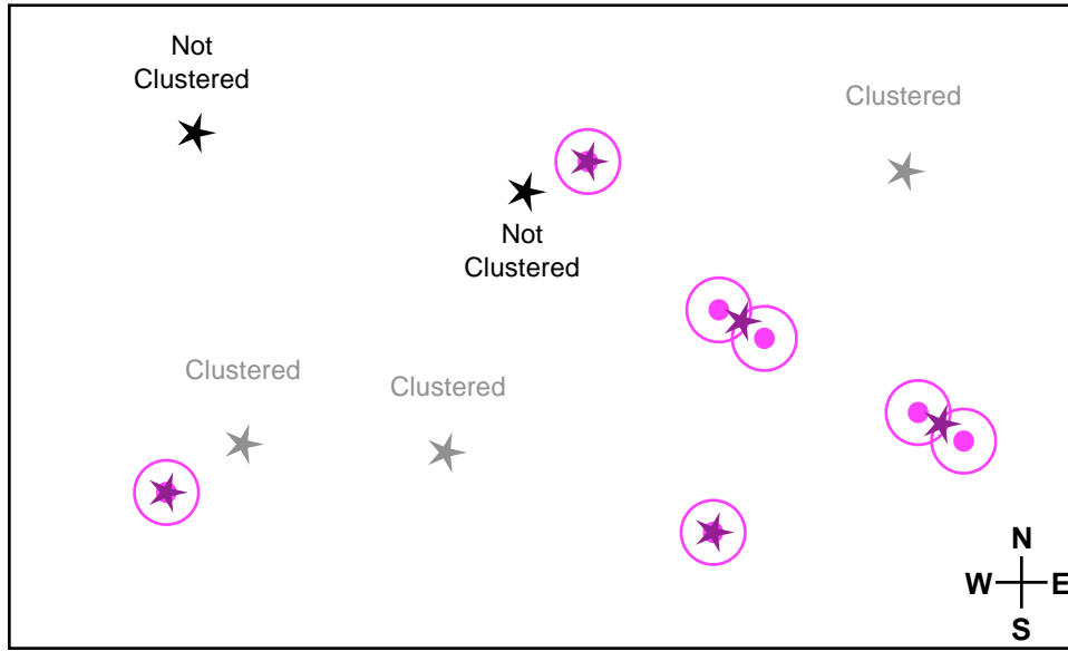
Figure 2.31: Step 3.c. Gray and black stars represent original group centroids labeled as “clustered” and “not clustered,” respectively, during generation of the Array master list in Step 1.
