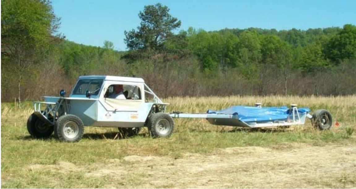
Figure 2.12: Photograph of the GEM Array collecting data at Camp Sibert.
