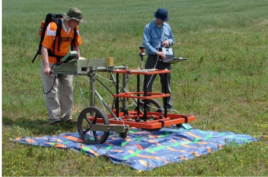
Figure 2.16: Photograph of the EM63 Cued collecting data at Camp Sibert. The instrument collected data along a grid drawn on a tarp that was laid over the cued location.
