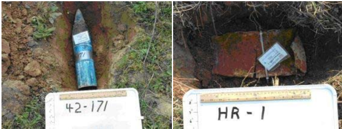
Figure 2.5: Photographs of an intact 4.2" mortar and a splayed half round seeded at Camp Sibert.
