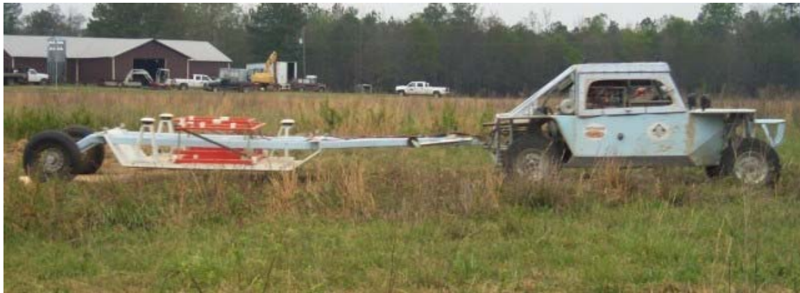
Figure 2.10: A photograph of the EM61 Array collecting data at Camp Sibert.
