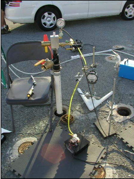
Figure 3-7. Modified Geoprobe® Pneumatic Slug Test Kit, capable of performing slug-in air vacuum tests
