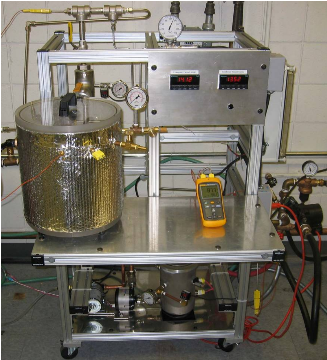
Figure 19. Overall Test Stand with Insulation and Updated Instrumentation
