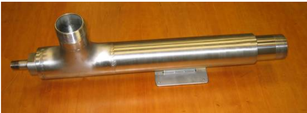
Figure 11. Custom Primary Ejector for Steam-Jet Chiller Evaluation
