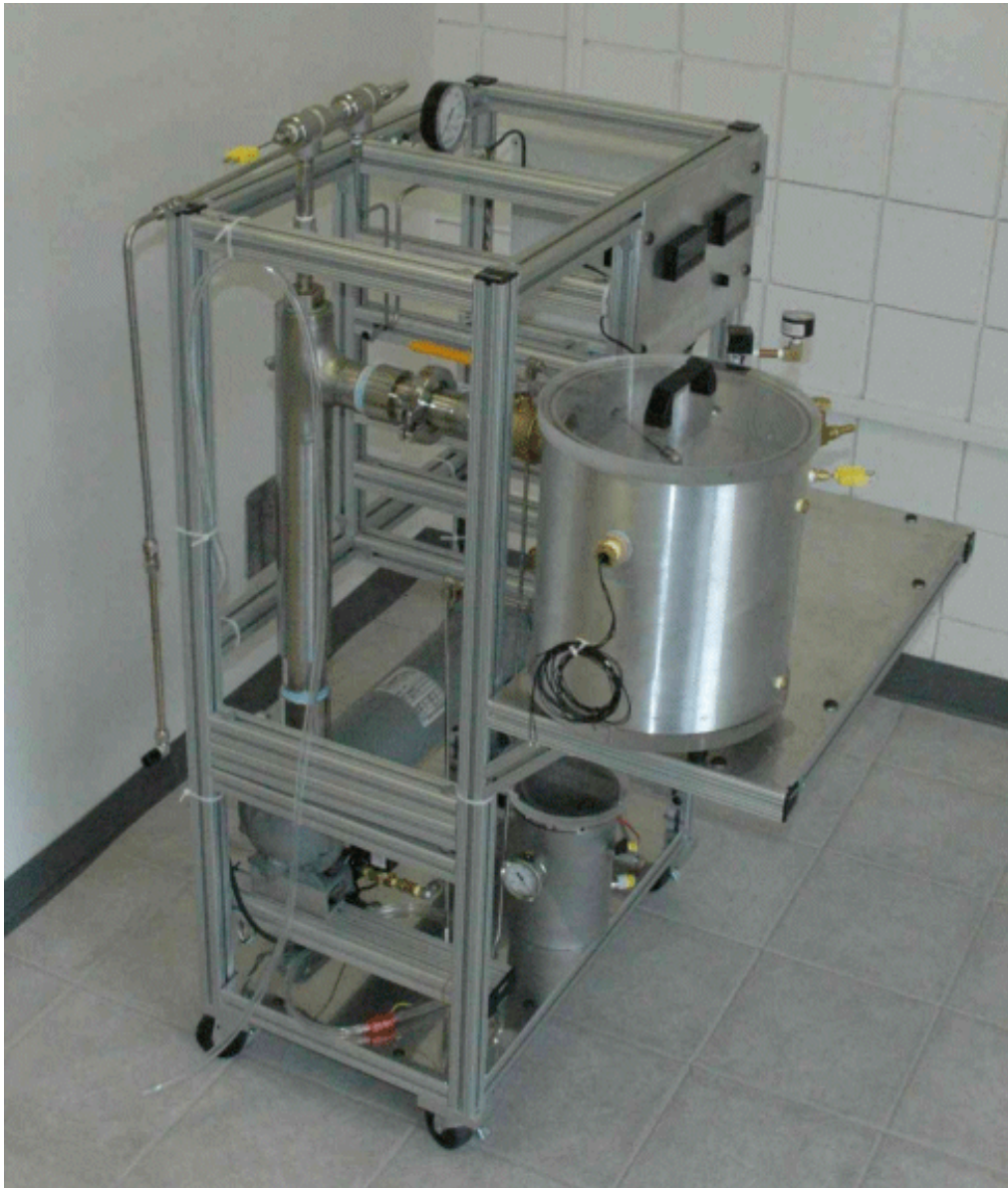
Figure 5. Steam-Jet Chiller Test Stand
