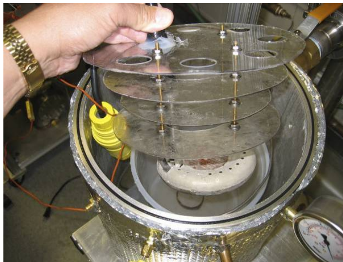
Figure 18. Heater and Baffles for Evaporator Chamber
