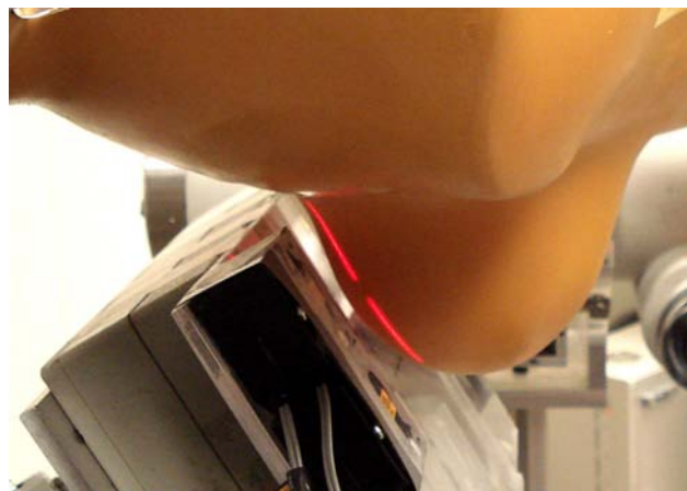
Fig. 7. (LEFT) Dual-layer prototype ribbon laser (Keyence Model HV300) contouring system attached to face of the SPECT camera. Sensor outputs are channeled through an ADC into the gantry motion controller (Newport ESP7000) that monitors and adjusts the ROR accordingly. (RIGHT) Separate 35 mm wide top-layer ribbon laser beams are seen on the breast phantom skin, as the camera dynamically contours at a minimal radius of rotation to improve resolution and image quality.
