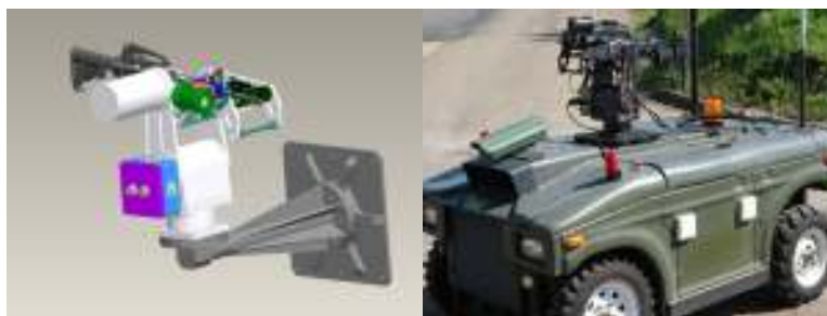
Figure 3. The NROWS System mounted on the MDARS UGV (right), and depicted in a wall-mount configuration.
