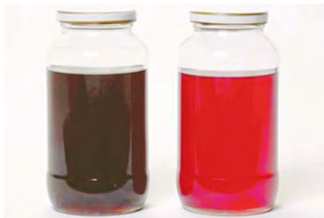
Sample results before (left) and after (right) fuel cleaning
