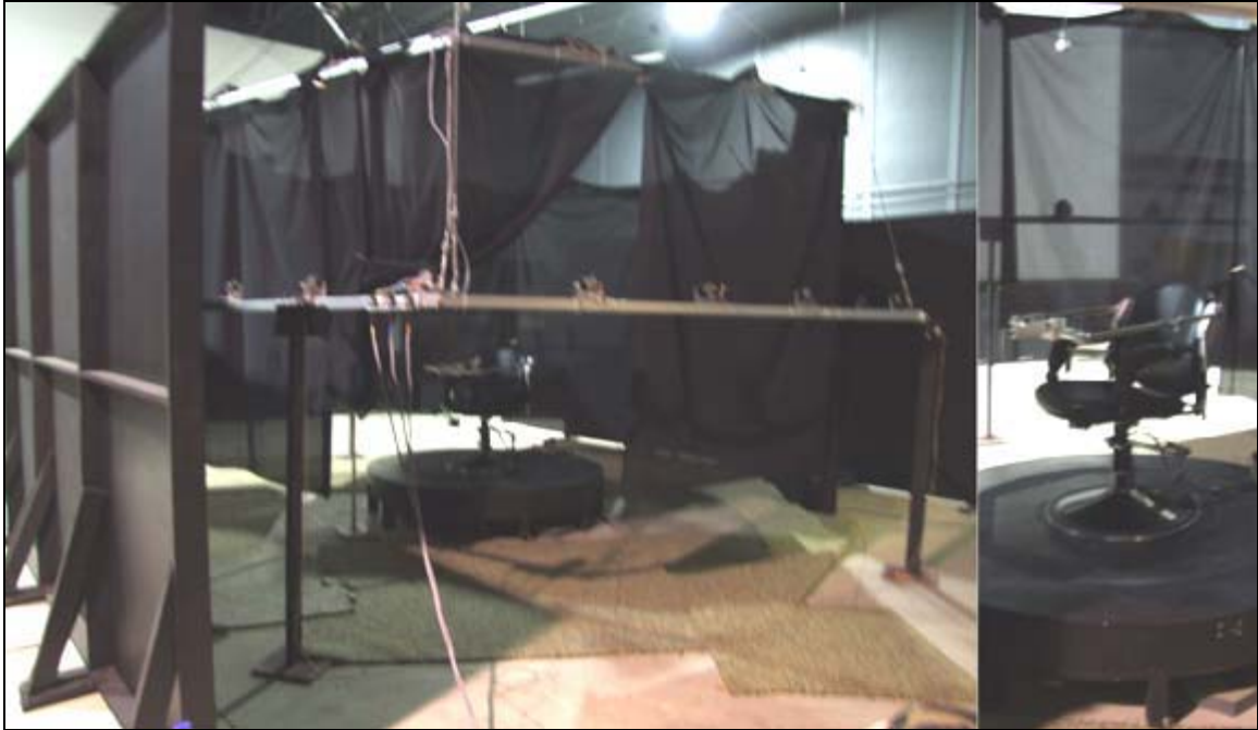
Figure 1. Test apparatus consisting of a suspended loudspeaker array, a rotating chair, and a digital pointing device. The curtains were used to hide the loudspeakers and the walls were used to create additional reverberation.
