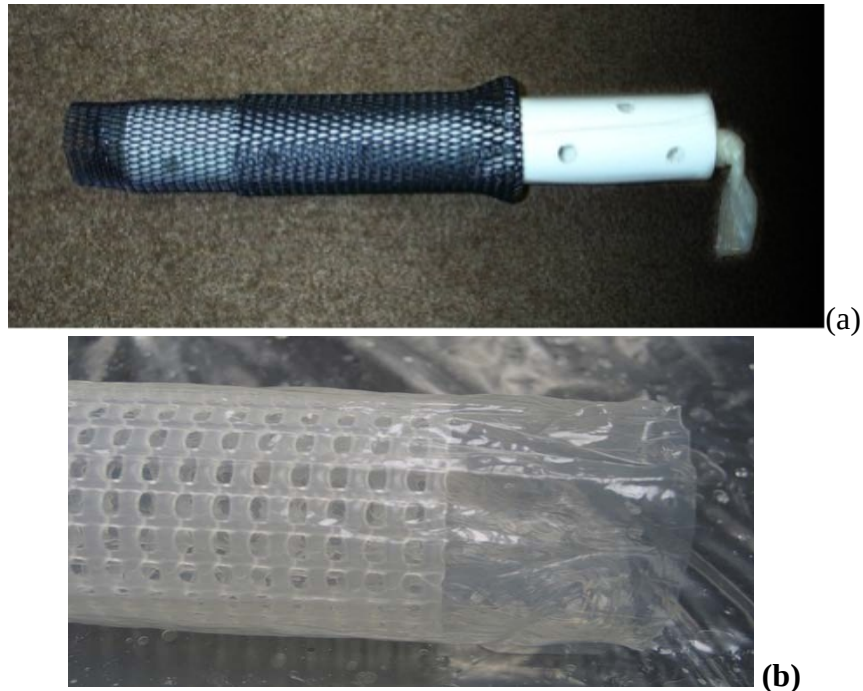
Figure 2-5. Regenerated-Cellulose Dialysis Membrane Sampler with Rigid Internal Support Made of (a) Perforated PVC and (b) LDPE Mesh
