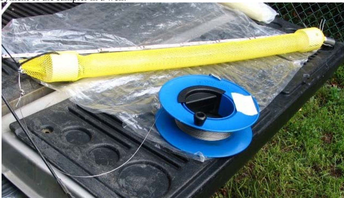
Figure 2-6. Example of Dialysis Sampler with a Plastic-Coated Stainless-Steel Suspension Line (2.5 inches in diameter by 36 inches long)
