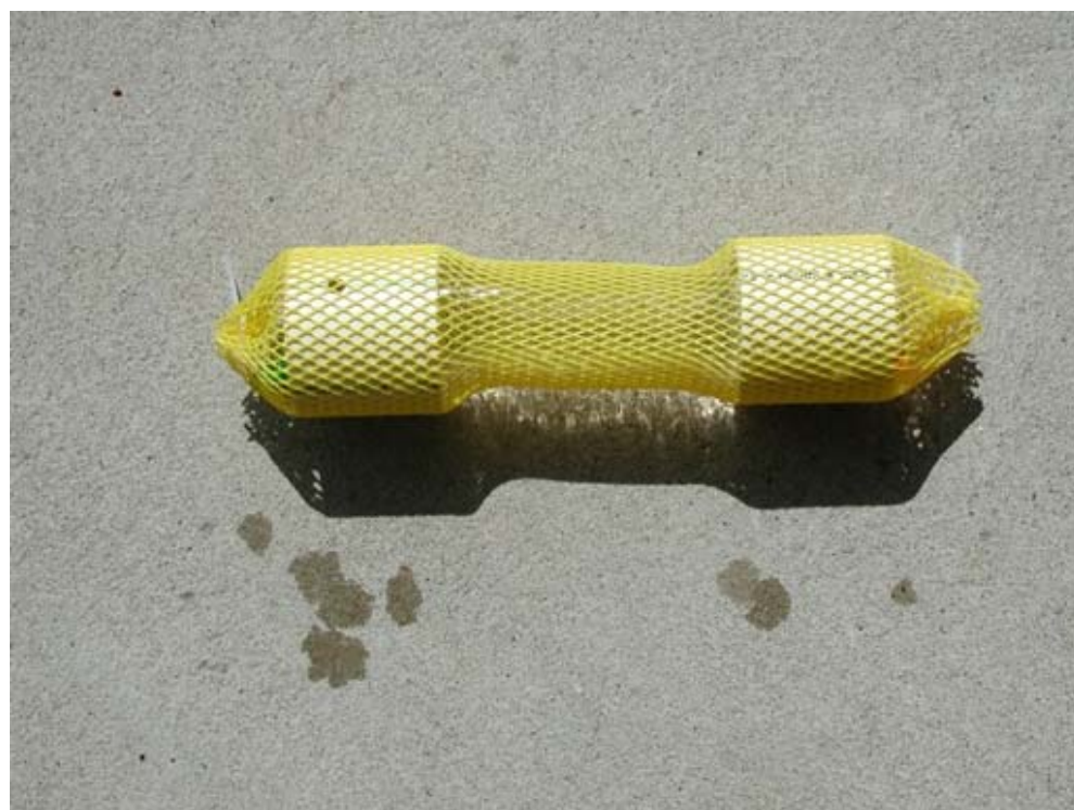
Figure 2-4. Fully Assembled Regenerated-Cellulose Dialysis Membrane Sampler with Supports External to the Dialysis Membrane (2.5 inches in diameter by 15 inches long)
