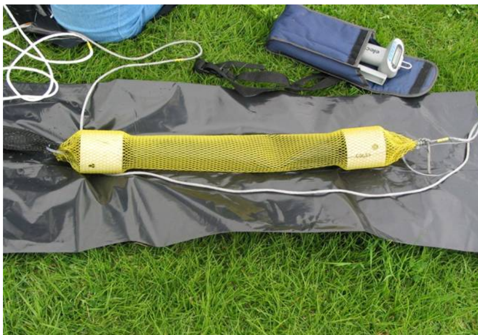
Figure 2-1. Regenerated-Cellulose Dialysis Membrane Sampler (2.5 inches in diameter by 24 inches long)
