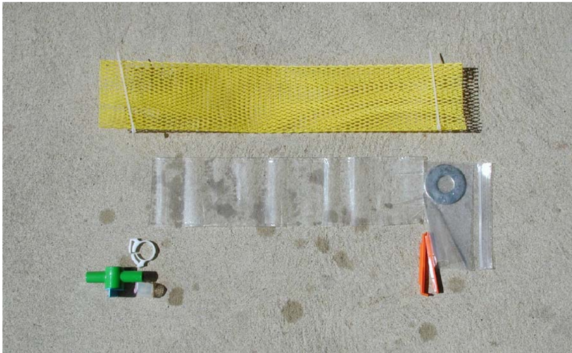
Figure 2-2. Disassembled Regenerated Cellulose Dialysis Membrane Diffusion Sampler, Showing Component Parts
