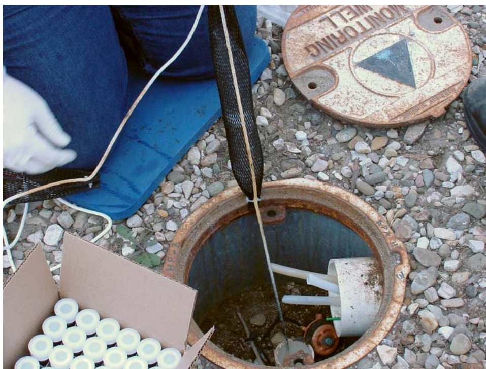
Figure 3-6. Removal Of Diffusion Sampler From A Well Prior To Sampling
