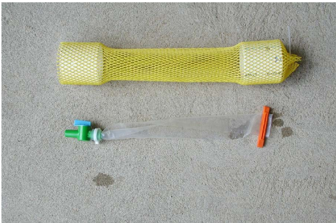
Figure 2-3. Partially Assembled Regenerated Cellulose Dialysis Membrane Diffusion Sampler, Showing Protective Mesh and PVC Pipe External to the Membrane
