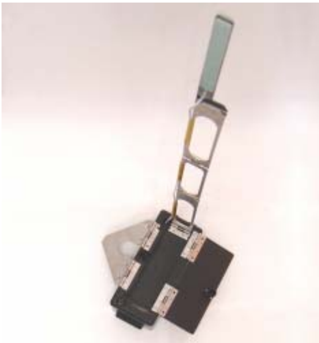
Figure 6. Relay Brick, shown as open and antenna mast extended.
