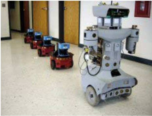
Figure 1. Convoy formation shown with SSC-SD's Robart III as the lead robot, followed by ActiveMedia Pioneer 2DX relay robots.
