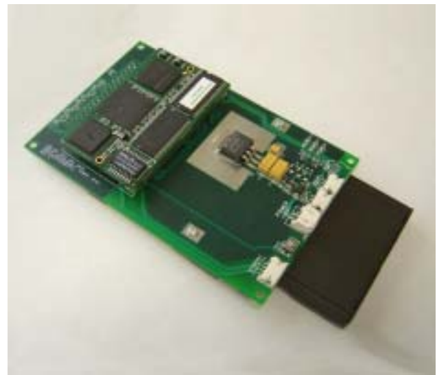
Figure 2. Top side of the CANR showing the nanoEngine, with the PC Card (bottom side) plugged into the RIB.
