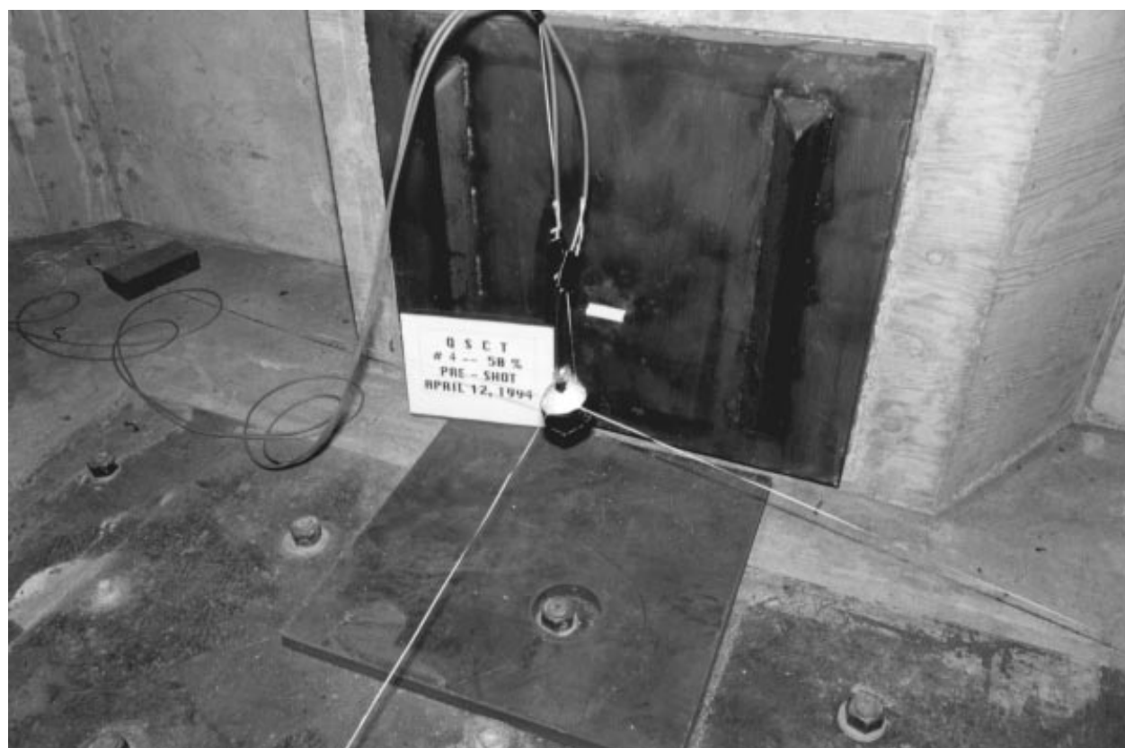
Figure 13. Explosive charge positioned in Zone 4 (near bullnose) prior to detonation.
