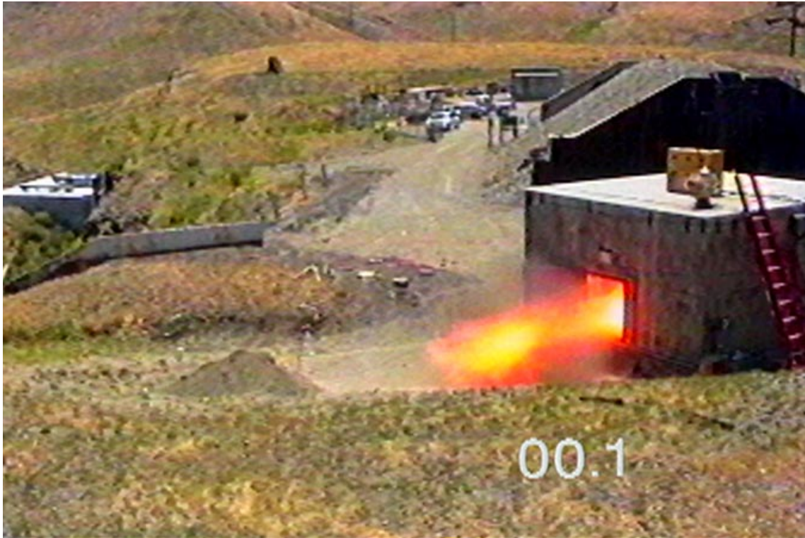
Figure 15. Double fireball recorded with 8-mm video camera during open-door test 15.
