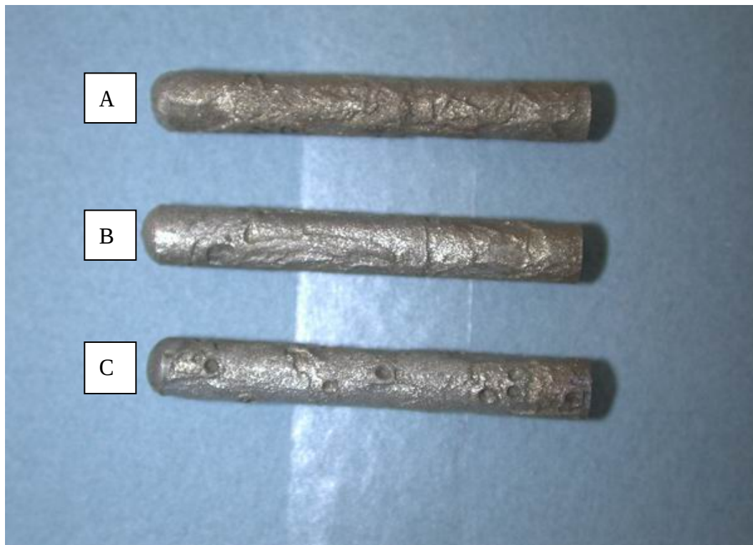
Figure 25. After-cleaning appearance of LPR probe electrodes from the raw water location (item C is freely corroding electrode).
