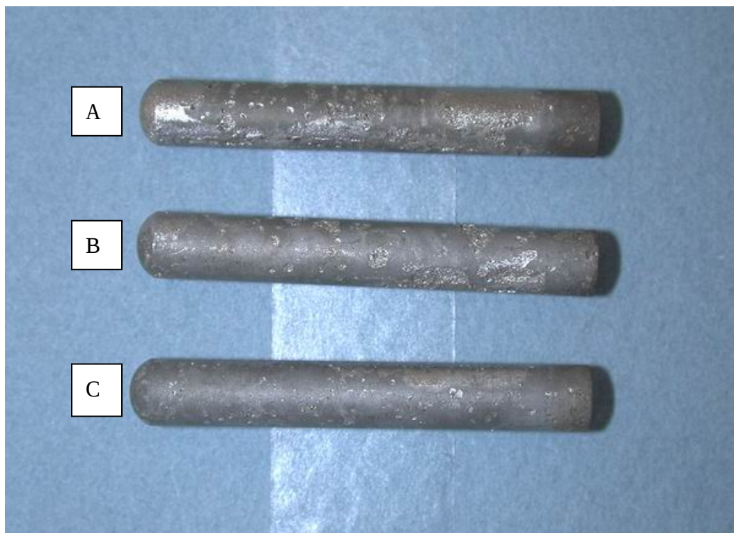
Figure 26. After-Cleaning Appearance of LPR Probe Electrodes from the treated water location (item C is freely corroding electrode)
