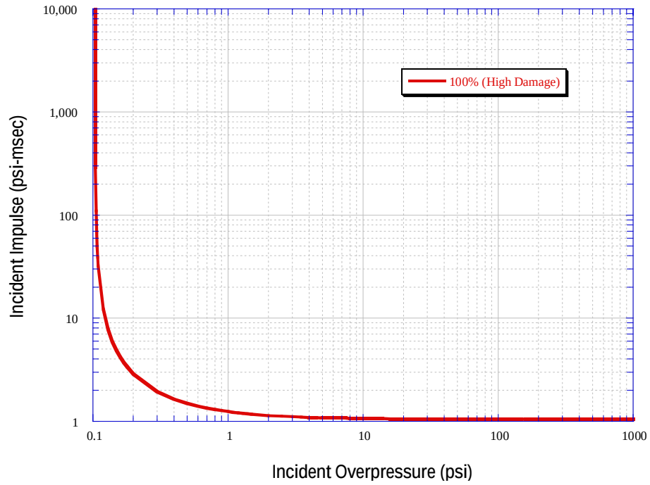
Figure 21. Gypsum / Fiberboard / Steel Joists Roof
