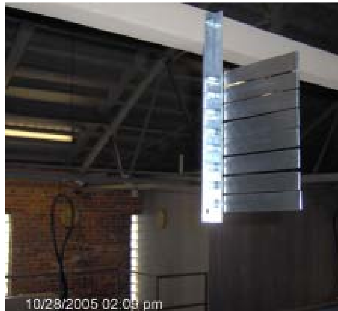
Figure 13a. Above water weight loss coupon at WTP.
