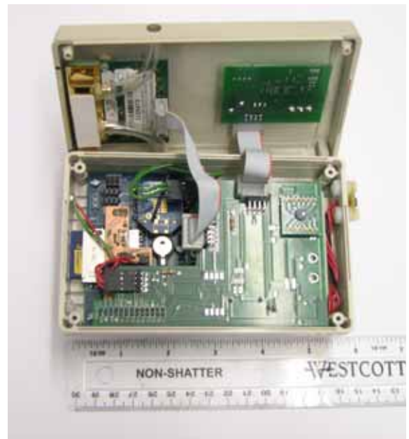
Figure 1b: Interior View of ASCENT 1000
