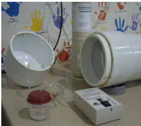
Figure 5. Altitude Chamber With CO 2 Calibration Gas
