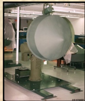
Ground Data Terminal (Line of Sight Link)
