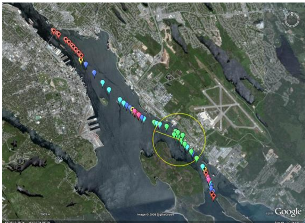
Figure 28: Locations of WiMAX data rate measurements plotted on Google Earth aerial photo. The symbol key is given in Table 3 and the yellow circle is 1 km in diameter (figure courtesy of David Williams, MDA).
