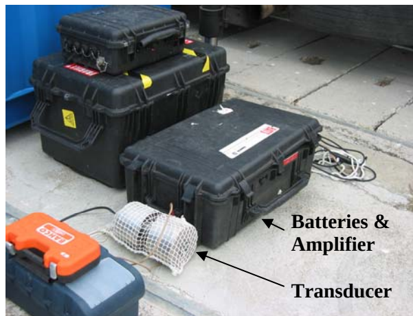
Figure 32: Broadband Acoustic Transmission System (BATS) used as a loud hailer.
