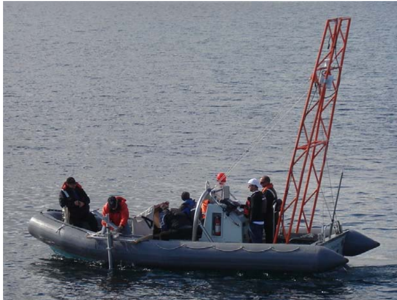
Figure 25: Barracuda 7-m RHIB outfitted as a response boat.
