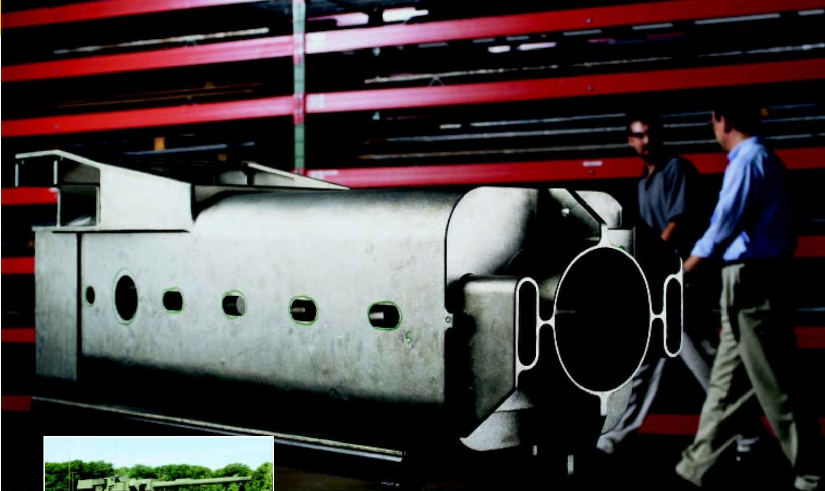
A titanium gun pod designed at the NCEMT will reduce the weight of the Stryker Mobile Gun System. Inset: Stryker Mobile Gun System under development by General Dynamics Land Systems.
