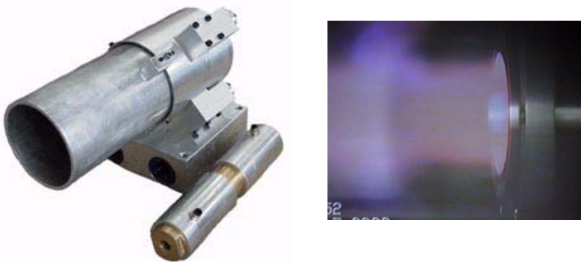
Fig. 17 – First airbreathing engine tested at LCD
