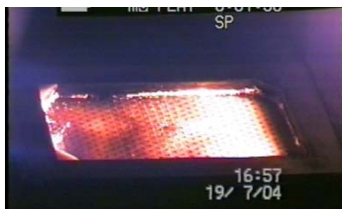
Fig.1 – Example of fuel-cooled panel tested in 2004
