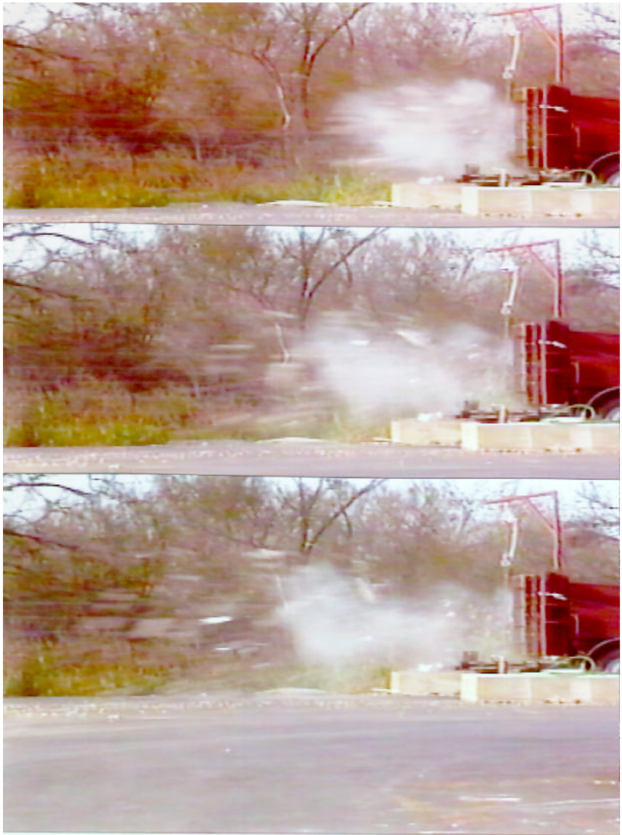
Figure 4. Debris From a Quarter-Scale Unreinforced Masonry Wall
