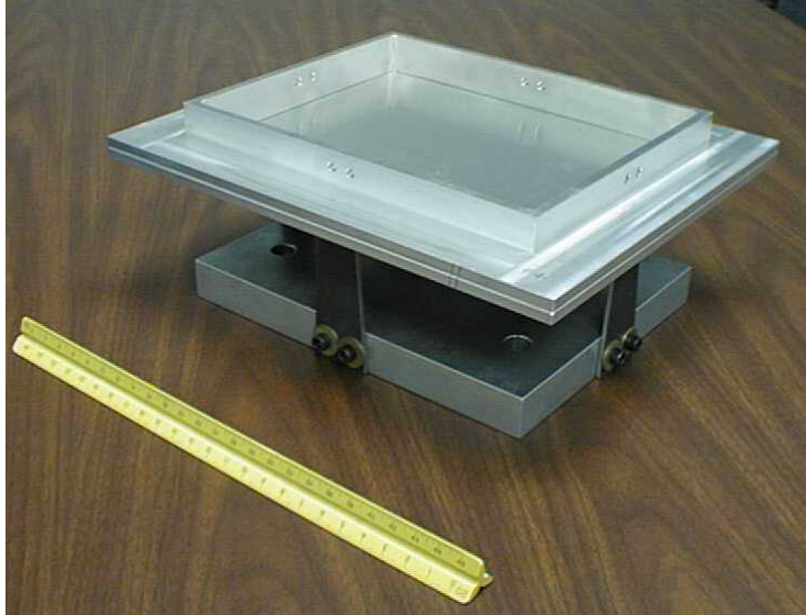
Figure 1. The test article shown mounted on flexures with a solid mounting plate.
