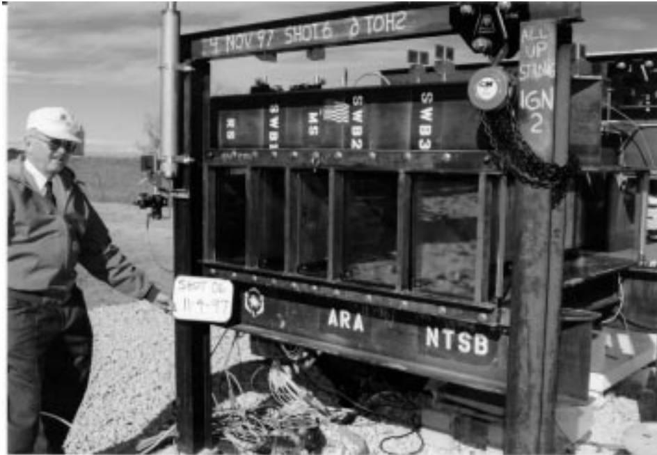
Figure 2. 1/4-Scale Test Fixture in Test Position
