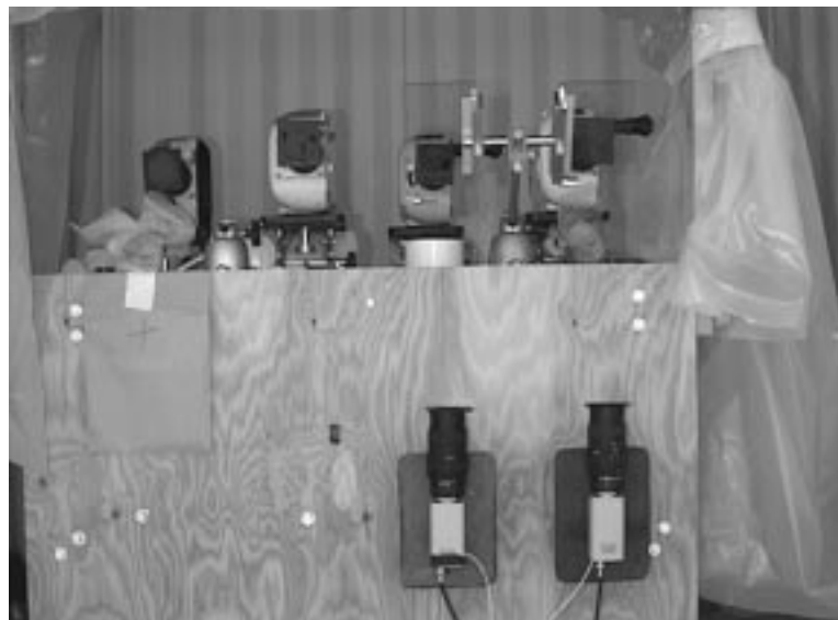
Figure 6. Combustion Photography Camera Station
