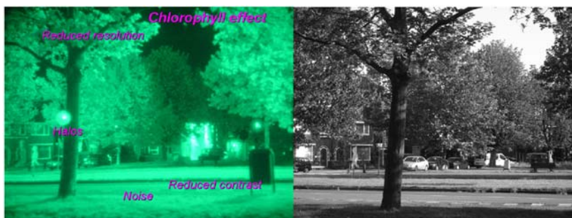
Figure 1. Demonstration of the differences between (right) black-and-white daytime images and (left) night-vision goggle (NVG) performance.
