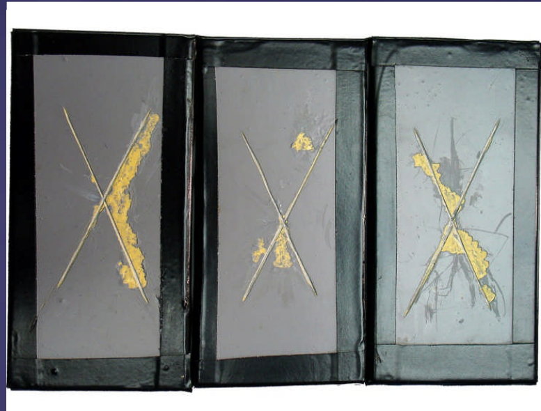
Primer (yellow) remains intact on Nanomyte PT-10 treated aluminum panels
