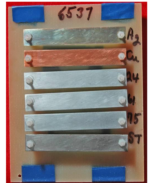
12 Month Indoor Exposure HMF Environmentally Controlled
