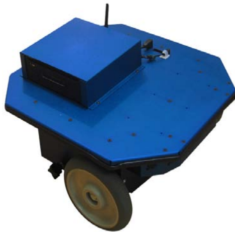
Figure 1. Base Model of the Erratic Mobile Robot [From 2].
