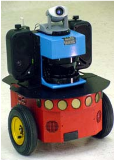
Figure 2. P3DX with Two-Dimensional Laser Mapping and Navigation and Complete Tracking, Vision and Surveillance Systems [From 3].
