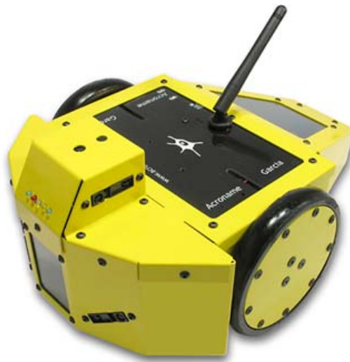
Figure 3. Base Model of the Garcia Robot [From 4].
