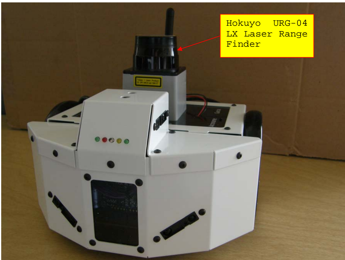
Figure 9. The Garcia Robot with the Hokuyo URG-04 LX Laser Range Finder on Top.
