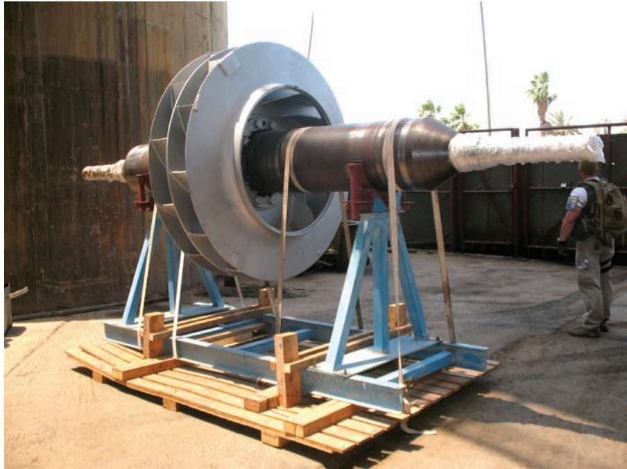
Rebuilt shaft for Unit 6 generator impeller.
