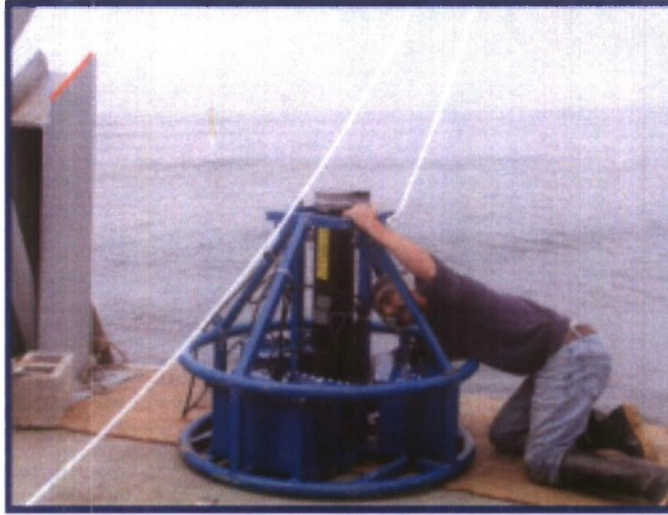
Figure A1-1: A TAPS-6 acoustical sensor is shown prior to its deployment at a station ca. 3.5 km SSW of Aptos, CA, near the 20 m depth contour. In this cage, a six frequency TAPS is mounted vertically (black cylinder). The LOCO sampling protocol required the TAPS to be configured as an up-looking echo sounder. A spar buoy can be seen floating in the distance. Data and power are transferred to a two-way VHF radio in the buoy via an electrical cable connected to the TAPS. Several key system parameters are programmable and were controlled from a shore station as needed.
