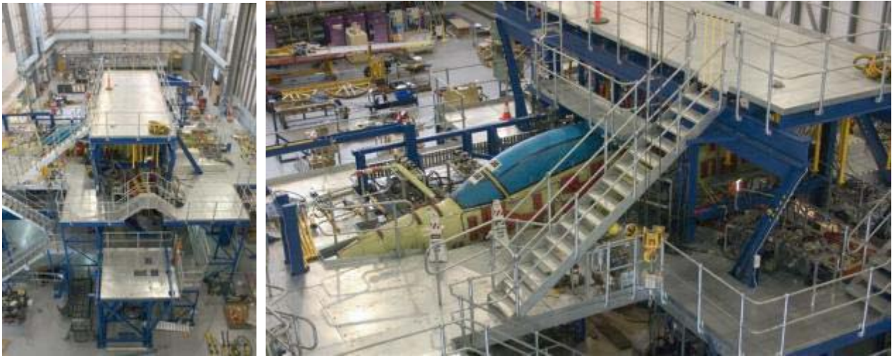
Figure 18 LIF Test Rig (left) under construction, and (right) with aircraft installed.
