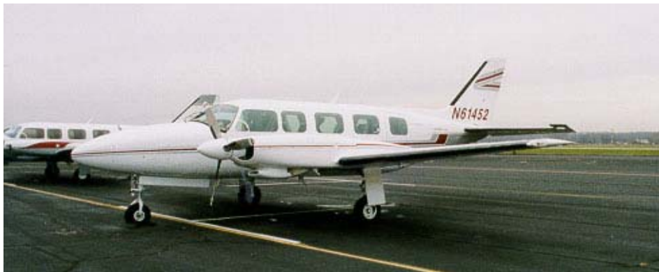
Figure 24 The Piper Chieftain has an Airworthiness Directive for fatigue management in Australia, but not in the USA
