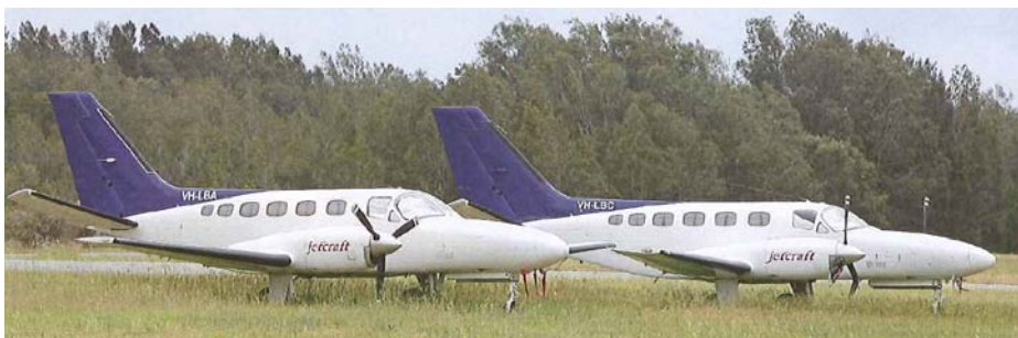
Figure 23 Cessna 441s that CASA grounded because they exceeded the LOV for their maintenance program
