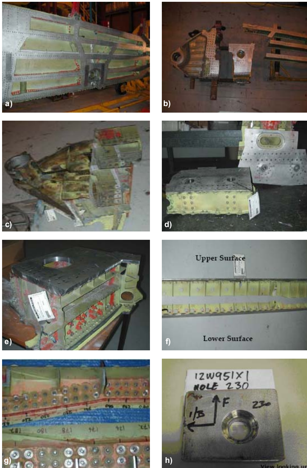
Figure 4 a) Upper Wing Skin removal; b) Separation of the Wing Pivot Fitting (WPF) and Inboard Pivot Pylon (IPP); c) WPF Lower Plate; d) Lower Wing Skin (LWS) Hardpoints; e) IPP Housing; f) Spar fragment; g) Example of water picked fragments; h) Fragment prior to being broken open for fractographic analysis.
