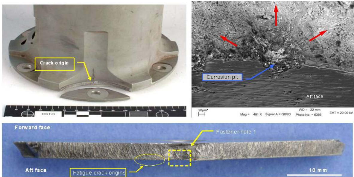
Figure 22 Black hawk high speed shaft tube cracking.
