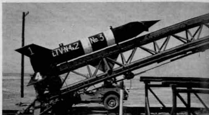
Rocket is shown on launching ramp. The rocket is fitted with a cone shaped dummy nose.
