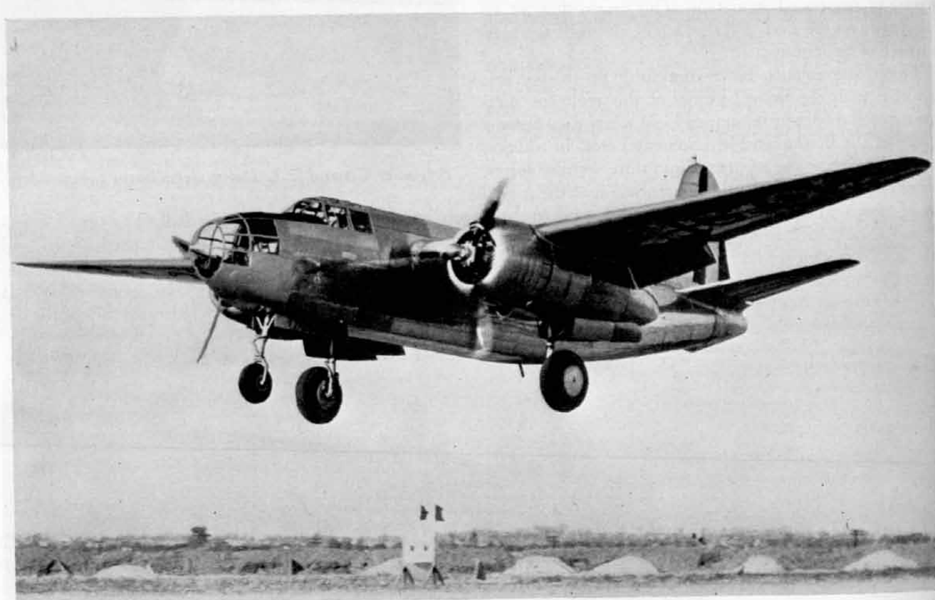
The attack bomber is a new and effective aerial weapon. The Douglas XA-20 attack bomber shown here is powered with two Pratt & Whitney 900-h.p. engines and is equipped with a tricycle landing gear.
